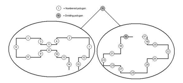
Figure 7. The result of a split at polygon 16
