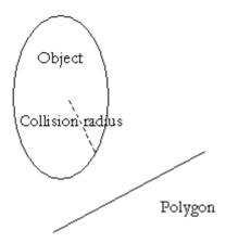
Figure 22. Collision radius.
